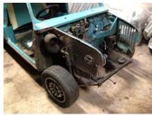
The front wings and front panel have been removed to evaluate what lies beneath! So far the passenger side flitch panel has been replaced as well as the door jamb. Next up should be the driver's side. More next month....
