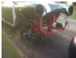
some pictures of his mini sporting a clam shell bonnet lift design (bonnet and wings having been welded together). The target is
